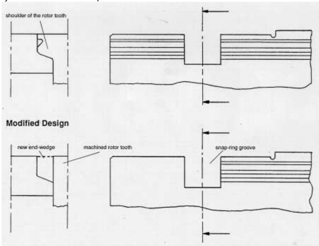
**Fig. 2: Comparison between the original design and the proposed modification. In the proposed modification the shoulders of the rotor teeth between the snap-ring groove and the end of the rotor body are machined off. The original end-wedges may be replaced by new end-wedges adapted to the new slot geometry.**
