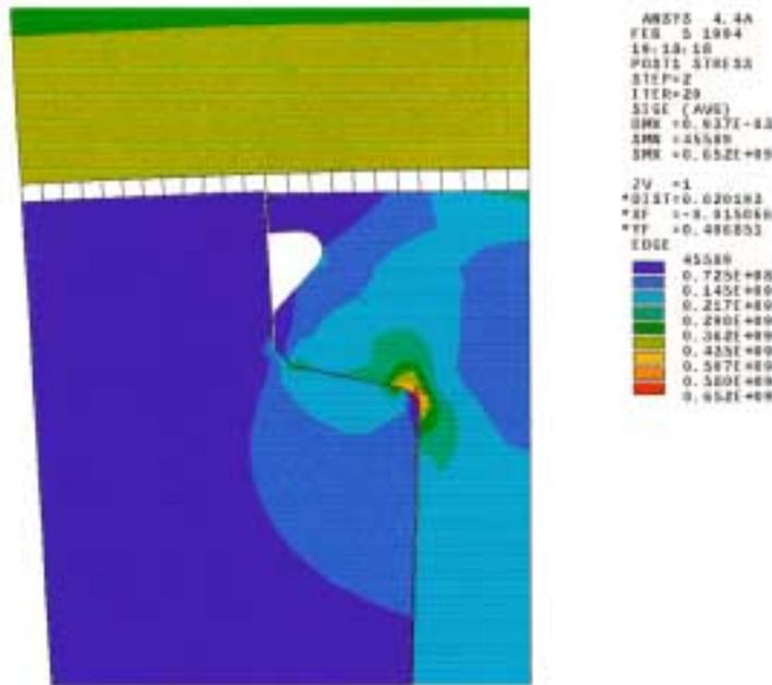
**Fig. 6: Equivalent elastic-plastic Mises Stresses (SIGE in N/m<sup>2</sup>) on a 40” rotor at rated speed. Highest stress is 94.6ksi.**
