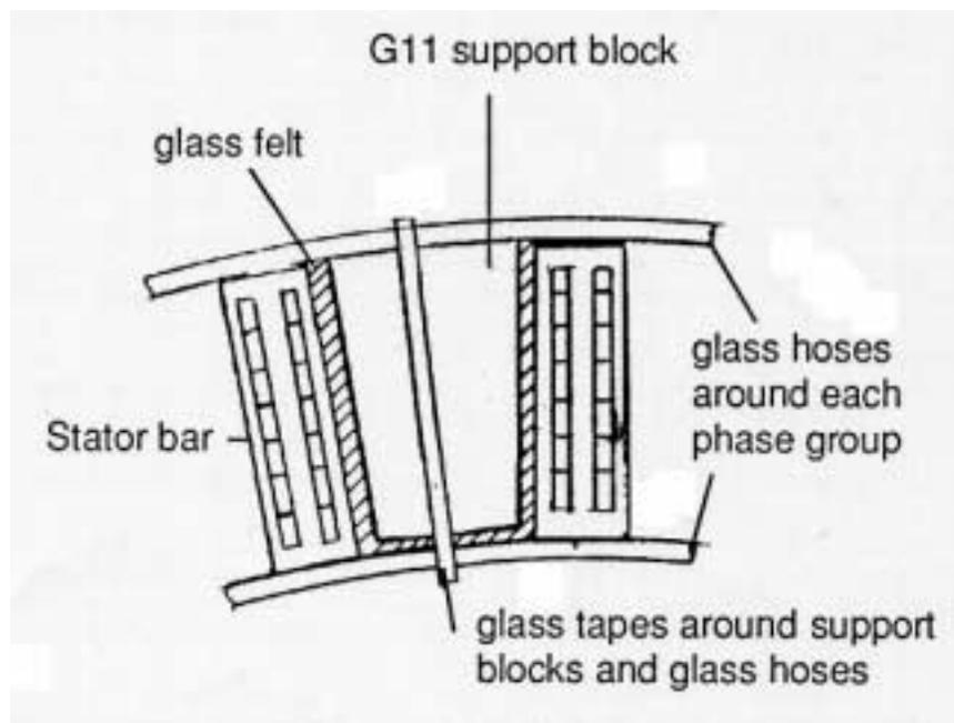
**Fig. 10: New circumferential blocking system.**
