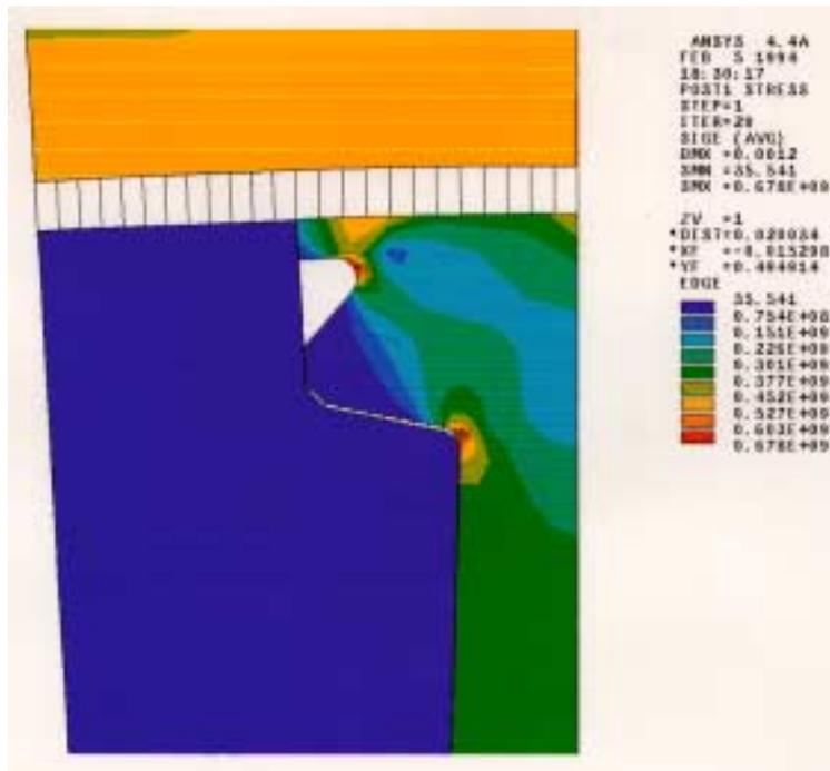
**Fig. 5: Equivalent elastic-plastic Mises Stresses (SIGE in N/m<sup>2</sup>) on a 40" rotor at standstill. Highest stress is 98.3ksi.**
