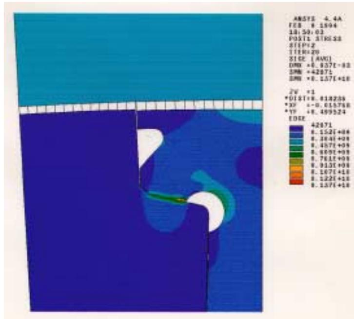
**Fig. 4: Equivalent elastic-plastic Mises Stresses (SIGE in N/m<sup>2</sup>) on a 40" rotor on the remachined rotor tooth at rated speed. Radius of the machined fillet is 0.1 inch. Highest stress is 198.7ksi.**
