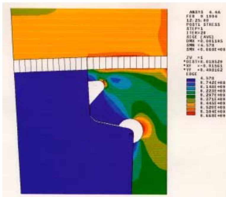
**Fig. 3: Equivalent elastic-plastic Mises Stresses (SIGE in N/m<sup>2</sup>) on a 40" rotor on the remachined rotor tooth at standstill. Radius of the machined fillet is 0.1 inch. Highest stress is 96.9ksi.**
