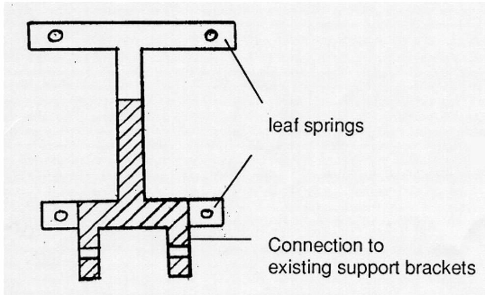
**Fig. 9: New support angles with axial flexibility.**
