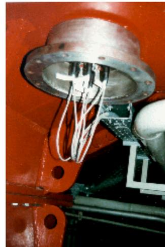
Fig. 5: Sealed Flange with Six Feed-through Conditioners and Cable
