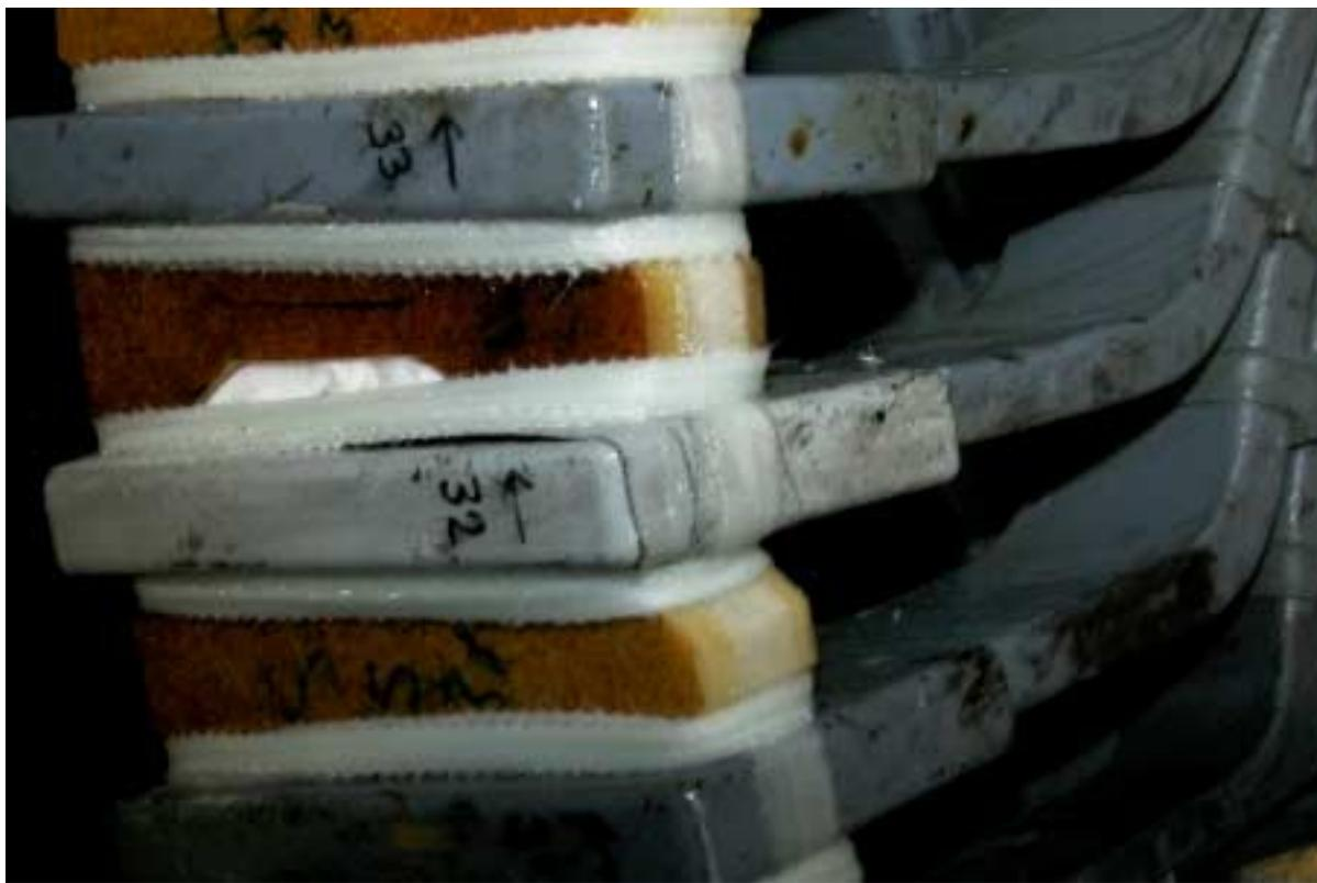
Fig. 11: Installed fibre optic accelerometer for tangential measurement
