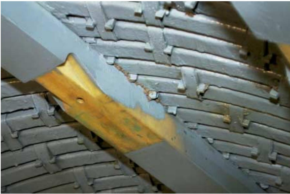
*Fig. 8: Insulation abrasion between end-winding support elements*
