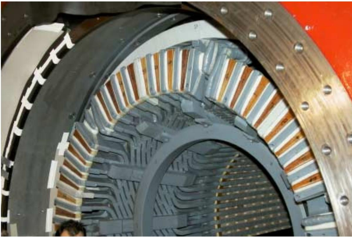
*Fig. 10: Example of tangential wedging of end-winding*
