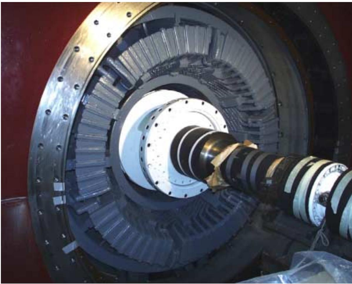
*Fig. 7: Hydrogen-cooled two pole generator (228 MVA and 15,5 KV stator voltage)*
